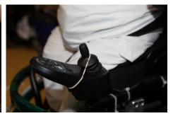
Please note that there is difference between the case that the joystick has moved from mid position to straight forward and the case that the joystick has moved little bit left or right and then straight forward. The Controlling Persons need to learn how to move the joystick without danger for the player.
