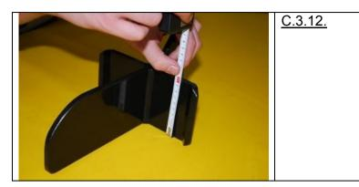
12. Width side wings is max.10 cm, measured from the blade.
